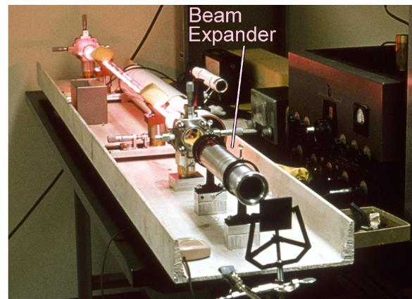
Fig. 1. 125- $\mu$ W HeNe laser used by the Electro-Optical Systems Amateur Radio Club in May, 1963 to transmit speech over a 190-km tropospheric path. The laser assembly, mounted in a steel channel, was externally excited using amplitude-modulated RF. Note the use of a beam expander.
