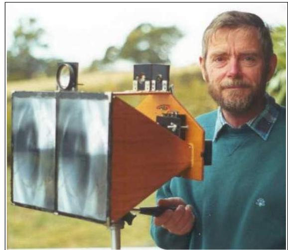
Fig. 9. A compact, truncated-pyramid optical transceiver using a pair of Fresnel lenses. Equipment like this has been used for two-way voice communications over 168-km (and longer) paths.
