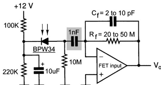
Fig. 11. "Daylight" modification of a transimpedance circuit to avoid DC saturation of the amplifier by photodiode currents.
