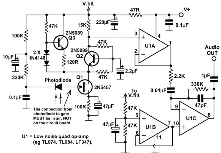
Fig. 14. High-sensitivity speech-bandwidth optical receiver.
