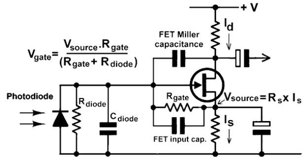
Fig. 13. The circuit of figure 12 with real-world leakage and parasitic components represented.
