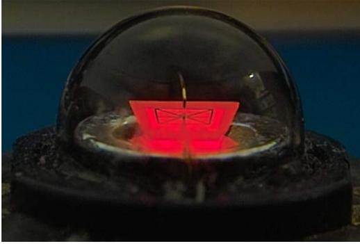
Fig. 5. A close-up view of a Luxeon III LED showing the dome, bond wire, and the TIP (truncated inverted pyramid) structure of the emitting die and its mounting on a reflective metal heat sink.
