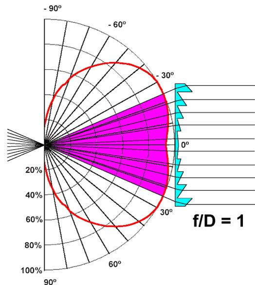
Fig. 7. Luxeon “Lambertian” polar pattern combined with Fresnel ray diagram. Only the portion that is shaded is collimated and over 65% of the LED’s output is wasted.
