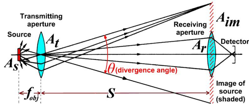
Fig. 3. Representation of a free-space optical system.
