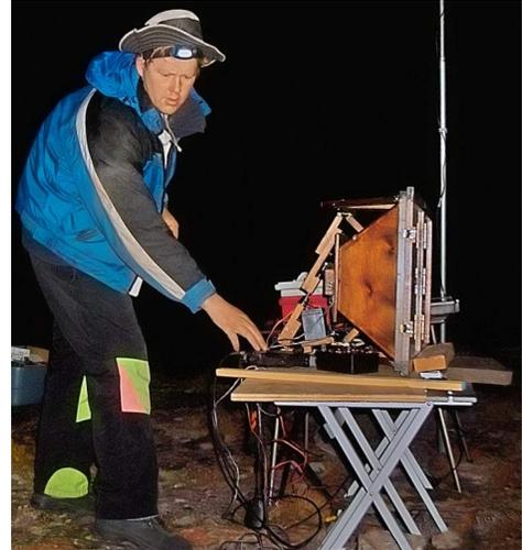
Fig. 2. Clinton Turner in October, 2007, at the north end of the 278-km optical path. This lightweight gear used inexpensive Fresnel lenses, a noncoherent light source, and despite rather poor seeing conditions, 2-way communication was established.
