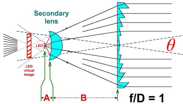
Fig. 8. Through the use of a secondary lens, more of the LED's output is intercepted and made available for collimation.
