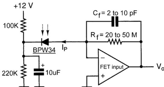
Fig. 10. A typical transimpedance (current-to-voltage) amplifier using a photodiode. The damping effects of the diode's capacitance are reduced as the low-impedance current input minimizes voltage changes.
