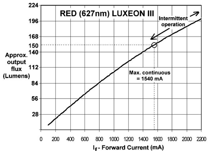
Fig. 6. Luminous output of Luxeon III versus current input for a red AlInGaP chip.
