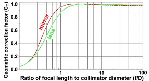
Fig. 4. The geometric correction factor  $G_T$ , plotted against collimator  $f/D$  ratio, for the radiation pattern of a “Lambertian” Luxeon III LED
