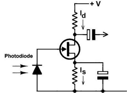
Fig. 12. High-impedance photodiode amplifier – the “K3PGP” circuit.
